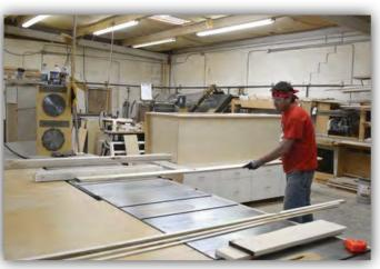
A bank of three vintage table saws is at the center of the shop. The saws are preset for various operations to speed conventional production.
