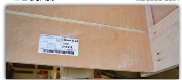
Using the Cabinotch system, all the cabinet components are fully labeled, making assembly fast and easy. The interlocking system allows for sure and speedy assembly.
